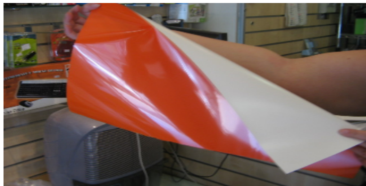
Illustrazione 2: glossy trasparent polyester on first face and white glue on second face
