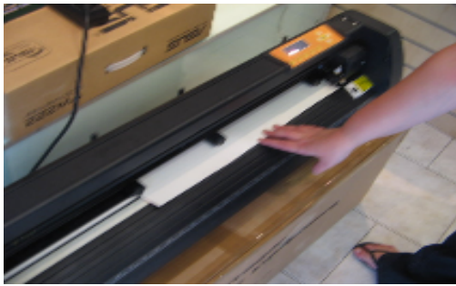
Illustrazione 3: positioning on cutting plotter, cut reverse graphics on white glue face
